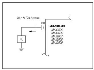
Figure 8. Inductive Reactance at Pin 1 (IND)
