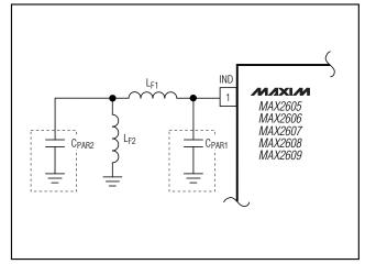
Figure 7. Simple Model of External Inductance
