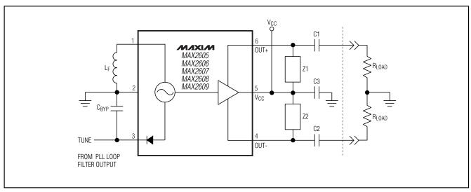
Figure 6. Typical Operating Circuit
