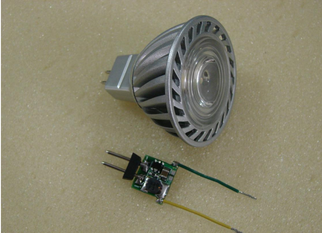
Fig 3 DEMO board for mass production
